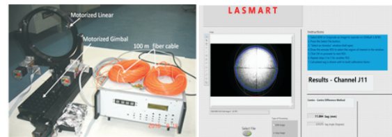
Fig. L.1.5: Motorized gimbal mounts and GUI of sag measuring software.
