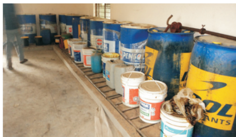
Fig. I.4.1: View of oil room with sand bed and oil drums.
