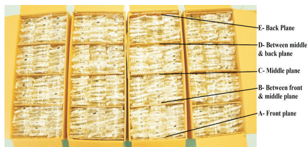
Fig. T.1.15: Volumetric dosimetry planes for dosimetry using electron beam from Linac-1.
