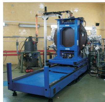
Fig. T.1.1: New 20 MeV injector microtron for Indus.
