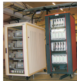
Fig. T.1.15: VME equipment control station to control active shunts for performing BBA.
