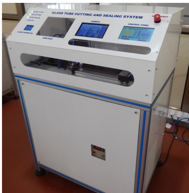
Fig. L.6.1: Glass tube cutting and sealing system.
