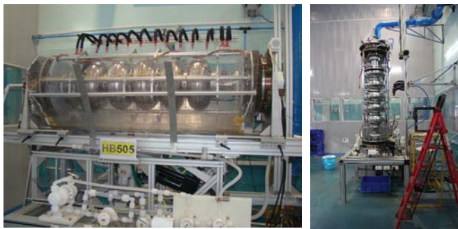
Fig. T.1.4: (a) Horizontal electropolishing setup for 5-cell cavity. (b) Setup in vertical orientation for acid draining and UPWrinsing.
