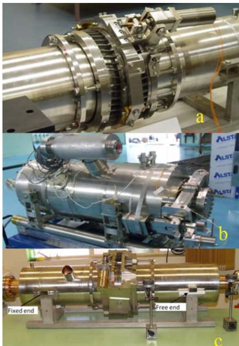
Fig. T.1.13: (a) Blade tuner, (b) Lever tuner and (c) X-link tuner.
