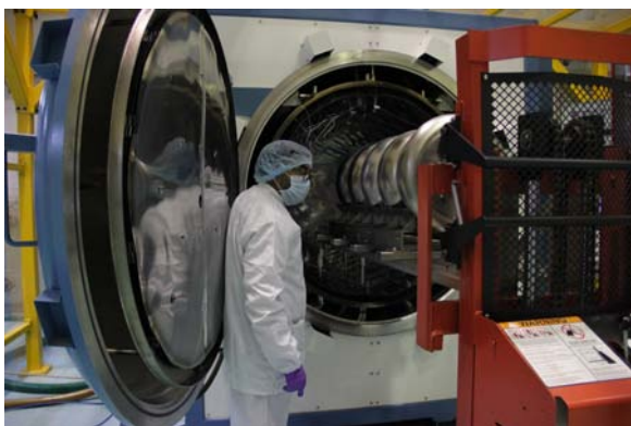
Fig. T.1.5: High temperature and high vacuum annealing of 5-cell 650 MHz SCRF cavity.
