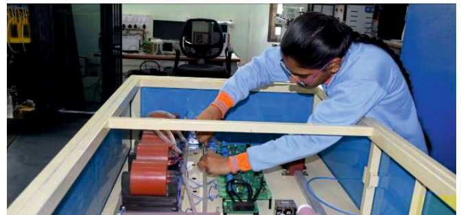
Apprentice performing electrical wiring of laser power supply.
