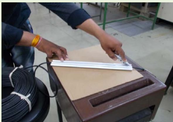
Fig. 34 Reuse of plastic sheath as protection jackets (1/2)
