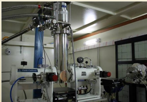
Cryostat mounted on stand at BL-09
