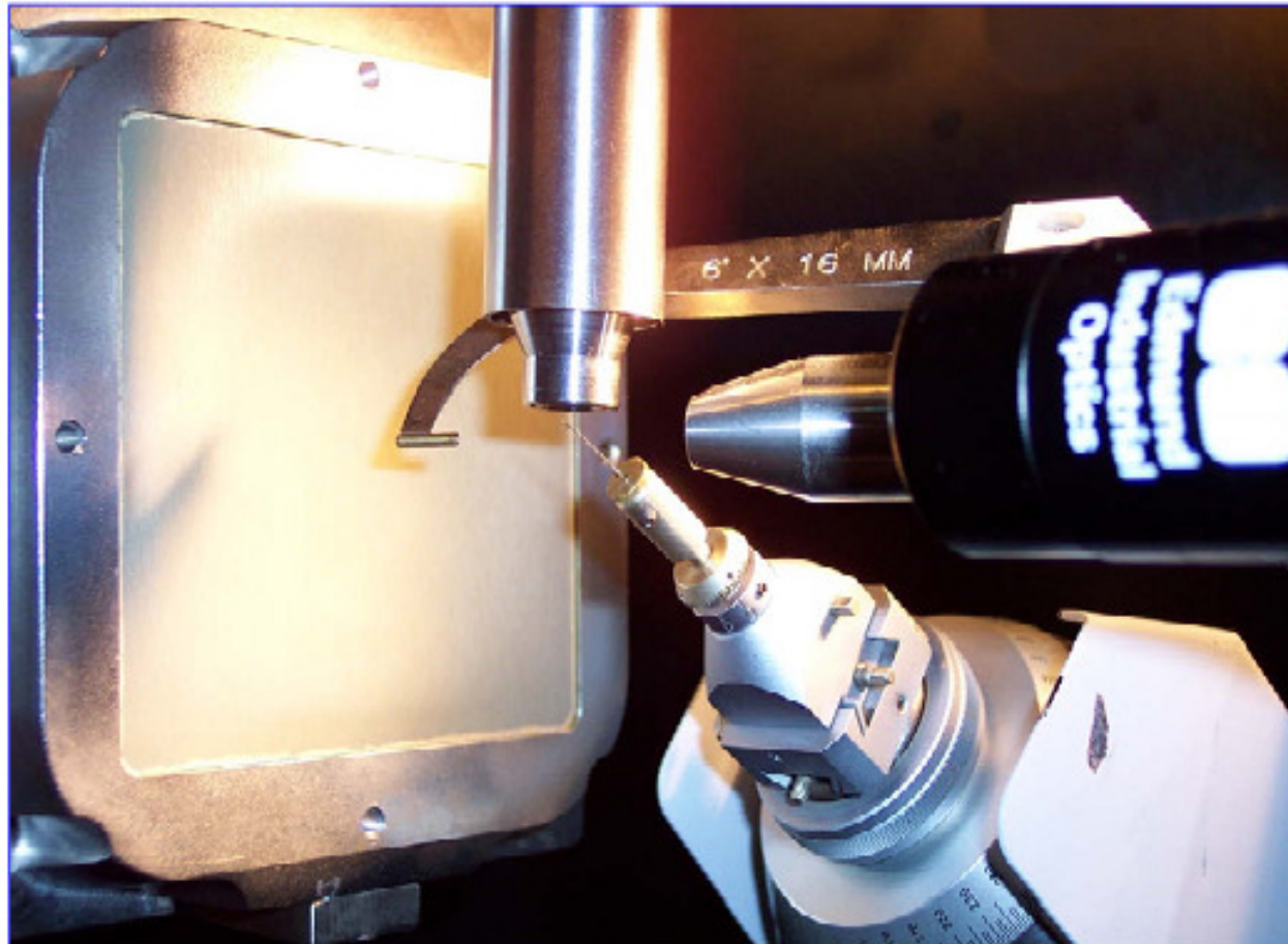
Figure 3: Bruker SMART APEX CCD area detector, Oxford nitrogen cryosystem, goniometer attachment with liquid mounted in a capillary.
