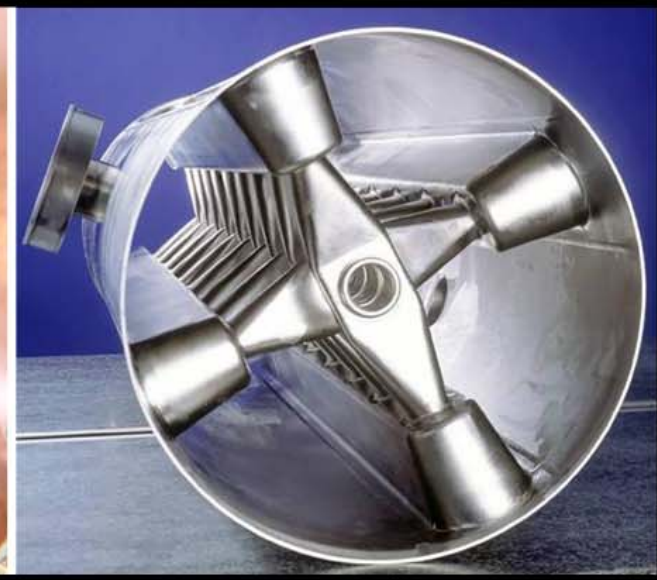
s.c. CH-DTL W < 150 MeV 150-700 MHz bulk niobium
