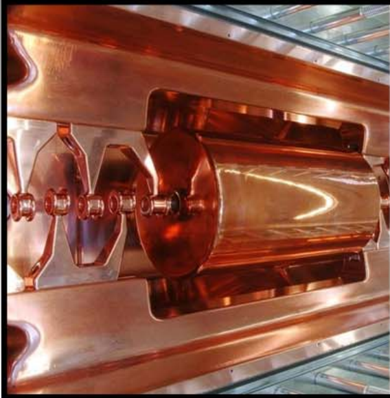
r.t. IH-DTL W < 30 MeV 30-250 MHz copper plated steel
