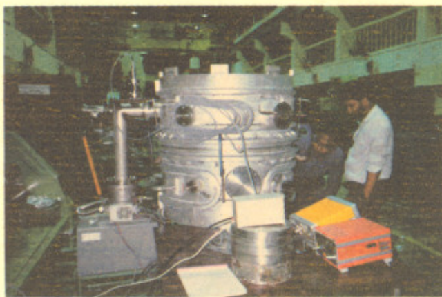
The RF cavity under inter-stage helium leak test during fabrication.
