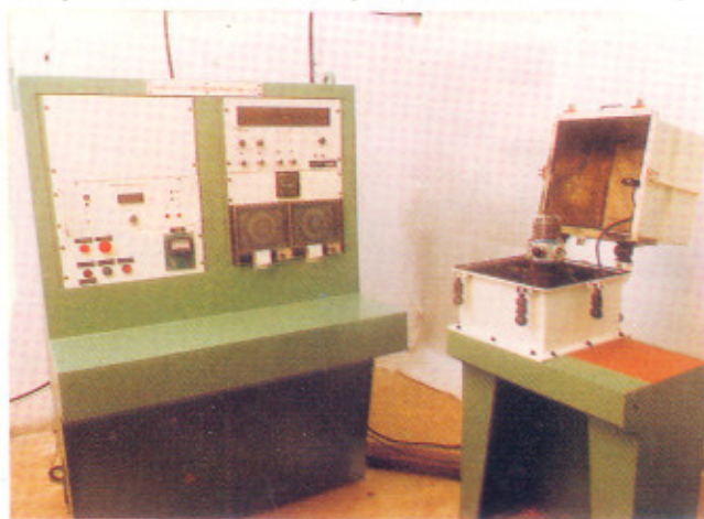
High-speed-assembly balancing machine for turbomolecular pump.
