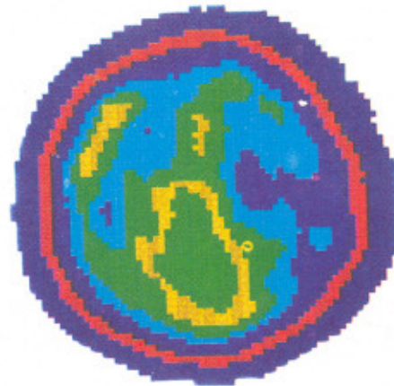
Near field spatial profile from VRM resonator configuration for Nd:YAG laser developed at CAT.
