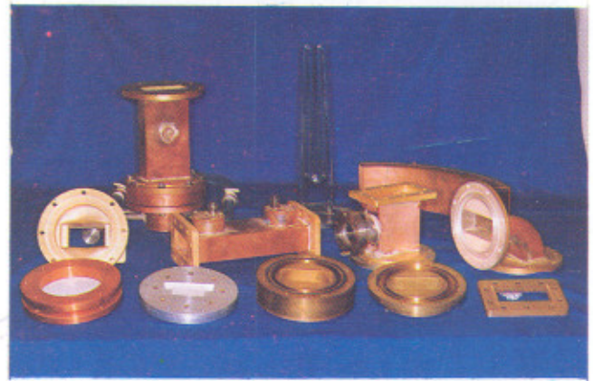
Various high power microwave waveguide components developed at CAT. Seen in the photograph are: microwave windows, dual directional couplers, circular to rectangular waveguide transitions, high power ceramic and glass type water load, vacuum wave guide section and bends.
