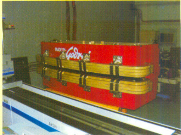
Fig.A.15.1 Prototype Dipole magnet with the CMM at the location of measurement.
