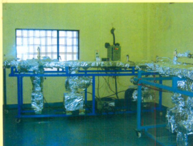
Fig. A.3.1 Assembly for baking of vacuum chambers
