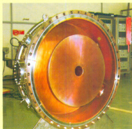
Fig. A.8.1 View of one half of the RF cavity
