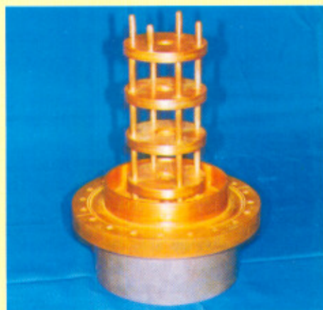
Fig. A.7.2 4-cell PWT linac structure
