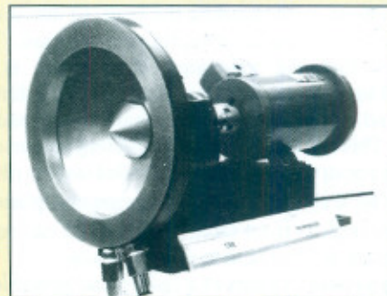
Fig. L.3.1 Rotating Water Cone Power Meter
