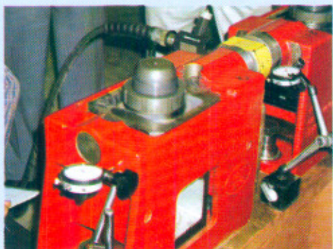
Fig.A.7.2 Two jacks under transverse load test
