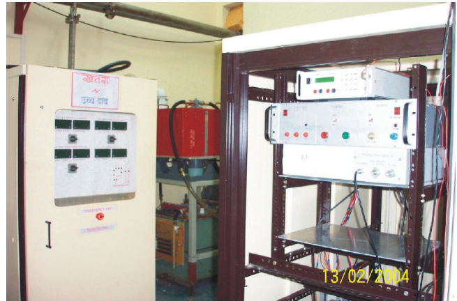
Fig. A.2.2 Photograph showing the 6MW peak, 25kW Average power microwave system developed at CAT for 10MeV LINAC
