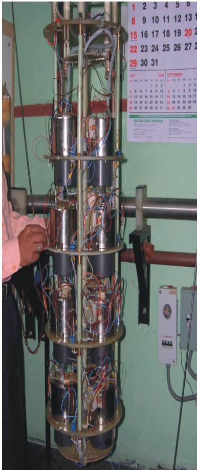
Fig.A.8.1 Showing 12 magnets on the test insert
