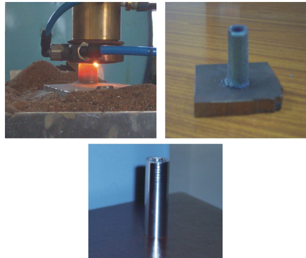
Fig. L.4.1 Different stages showing laser rapid manufacturing of Colmonoy bush
