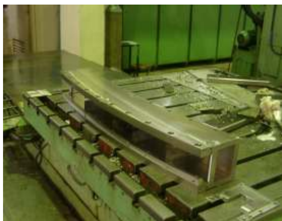
Fig A.6.2 Magnet body during machining at HBM-AZ-11
