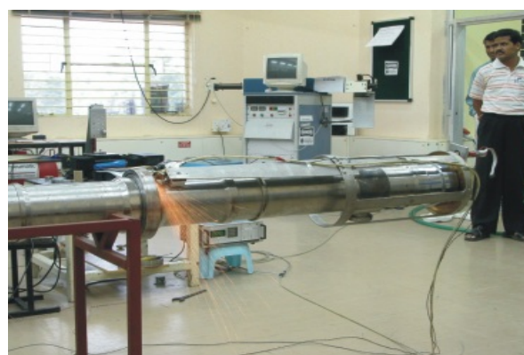
Fig. 18.L.1 Bellow lip cutting demonstration
