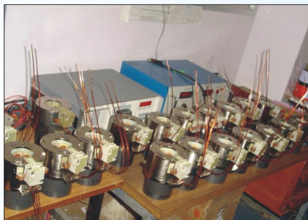
With the despatch of last batch of Sextopole Corrector Magnets CAT completed this supply to CERN. The cryogenic and magnetic field quality testing of these magnets was also done at CAT.
