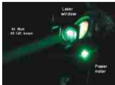
Fig. L.7.1 94 watt CVL beam being coupled out from laser window.
