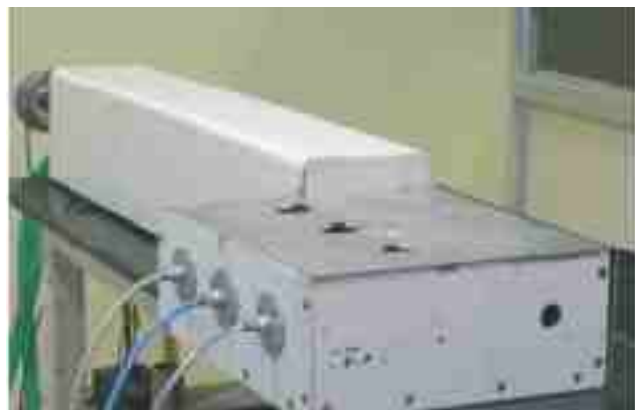
Fig. T.3.1: Industrial Nd:YAG laser with time-shared fiber-optic Beam delivery.
