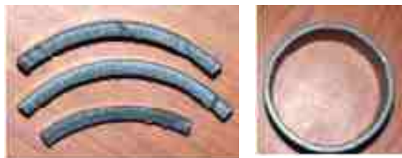
Fig.T.3.11 shows cut samples from pressure tube.
