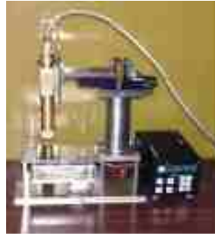
Fig. T.3.14(a): Brachytherapy capsule welding fixture.
