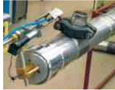
Fig.T.3.4: Fixture mounted on coolant channel for laser cutting of HPFC studs.
