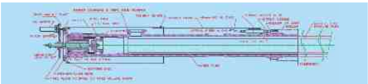
Fig.T.3.3: A sketch of bellow lip cutting fixture mounted on E-face of coolant channel.
