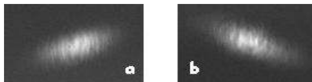
Fig.L.3.2: Typical AC traces for the case of (a) a single prism; (b) a pair of prisms
