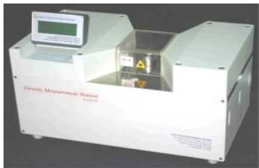
Fig.T.1.5: Density measurement station.
