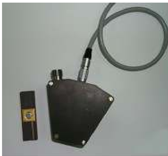
Fig.T.1.7: The laser triangulation sensor developed for position sensing applications.
