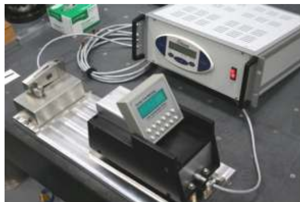
Fig.T.1.6: Nuclear fuel metrology system for mixed carbide fuel.
