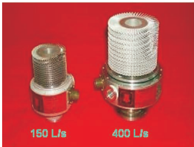
Fig..A.7.1: Assembly of turbomolecular pumps
