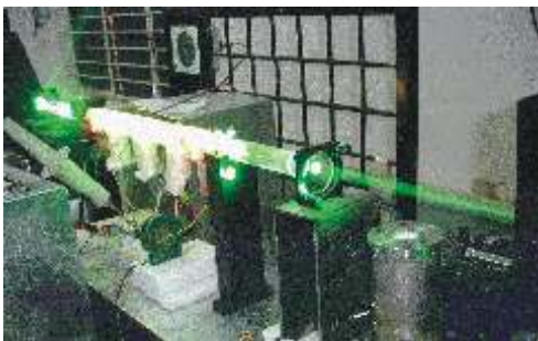
Fig.L.8.2 : Photograph of the sealed-off CuBr laser
