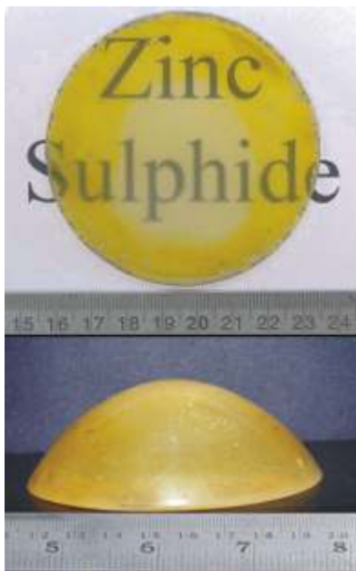
Fig.L.12.2 Stand-alone ZnS after polishing in different shape
