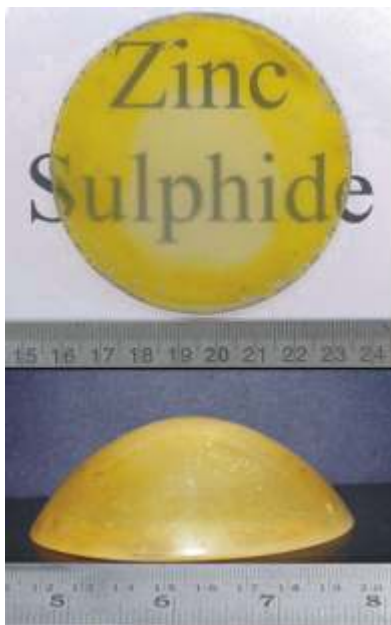
Fig.L.12.2 Stand-alone ZnS after polishing in different shape
