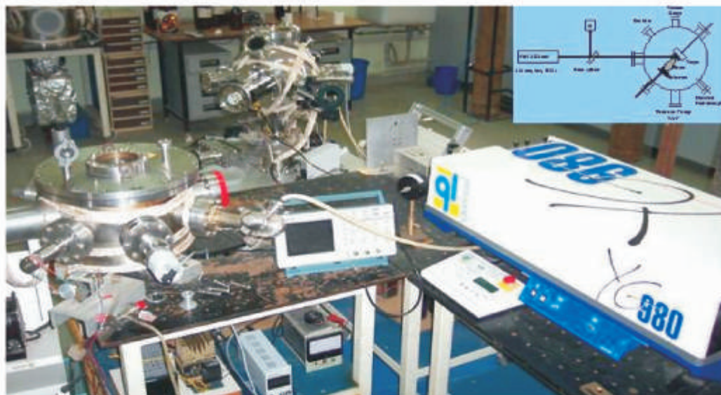
Fig. T.1.2: Pulsed Laser Deposition system. Inset shows the schematic diagram of this system.
