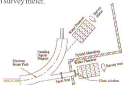
Fig.T.3.4: Schematic diagram of the experimental set-up for depth dose measurements.
