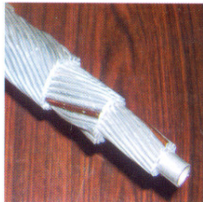
Fig.A.9.1: Water-cooled stranded cable, showing strands in various layers.
