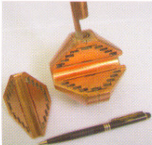
Fig.A.5.1 Cut view of the six-channeled drift-tube.
