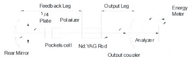
Fig. L.11.2: Resonator with the Pockels cell kept after the polarizer and before the \lambda/4 plate in the feedback leg
