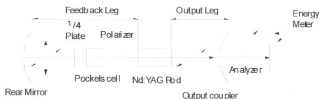
Fig. L.11.2: Resonator with the Pockels cell kept after the polarizer and before the \lambda/4 plate in the feedback leg
