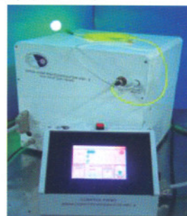
Fig.T.2.10: A photograph of the photocoagulator system based on diode-end-pumped intracavity frequency doubled green laser
