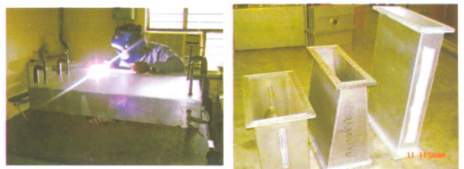
Fig.A.8.3: Some of the WR 2300 waveguide components viz., straight FH and HH sections, coaxial to waveguide transitions, F/H taper transitions, developed at RRCAT.(courtesy Mr. A.K. Jain, Mr. S.D. Sharma, Mr. V. K. Bhatnagar, ACEPD).
