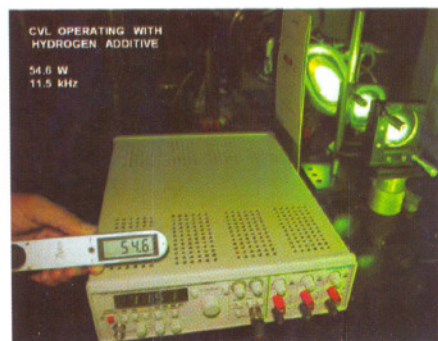
Fig.L.3.3. CVL operating with hydrogen additive delivering 54.6 W at 11.5 kHz rep-rate
