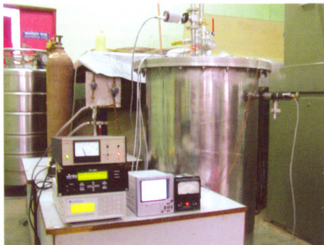
Fig. A.11.2: Experimental setup with 2 K cryostat
