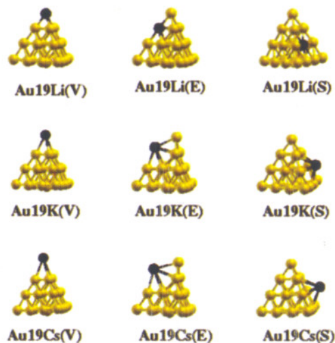
Fig. T.2.8 : Some of the gold clusters, with a replacement doping of one alkali metal atom. V, E and S represents vertex, edge and surface sites of the gold cluster. Li=Lithium, K=Potassium, Cs=Cesium.
