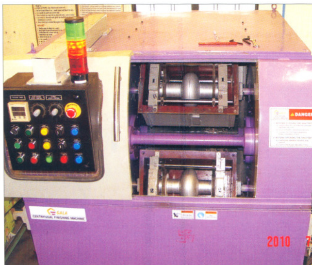
Fig. A.9.1: Barrel polishing machine for Single cell 1.3 GHz SCRF cavity.
