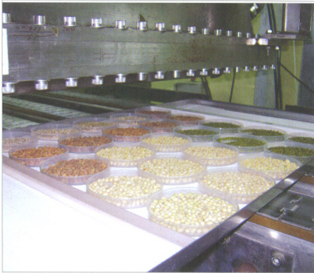
Fig.A.10.1: The irradiation system during dosimetry qualification using B3 film. Also seen in the picture is the beam scanner and conveyor system.
