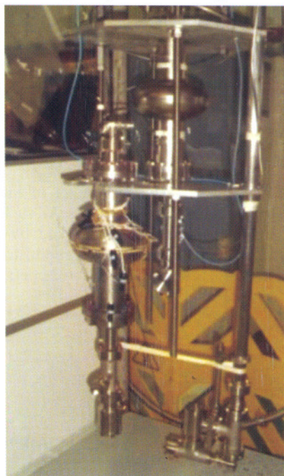
Fig.A.8.1: The single cell SCRF cavities mounted in VTS for 2K test at FNAL.
