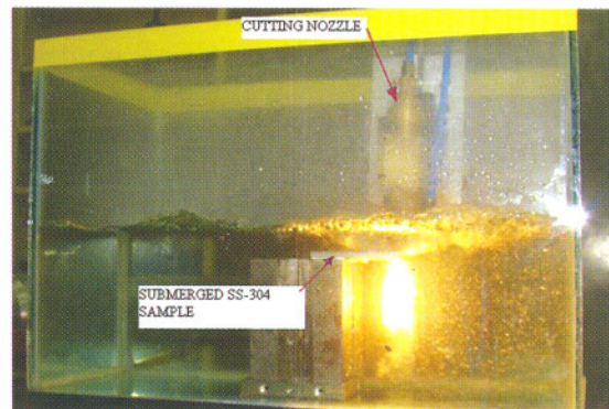
Fig. L.10.2: A view of underwater laser cutting of SS304.
