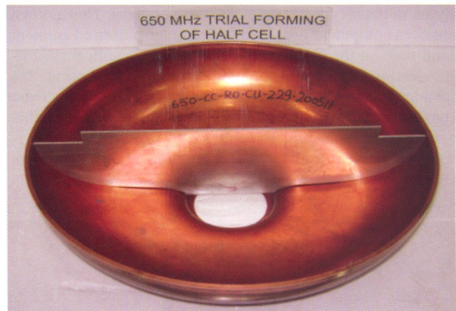
Fig. A.11.4: Formed half cell-inside view with inspection template also in view.
