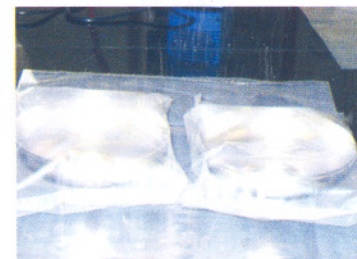
Fig. A.4.2(d): Packing in inert atmosphere
