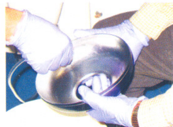
Fig. A.4.2(c): Drying with pure nitrogen
