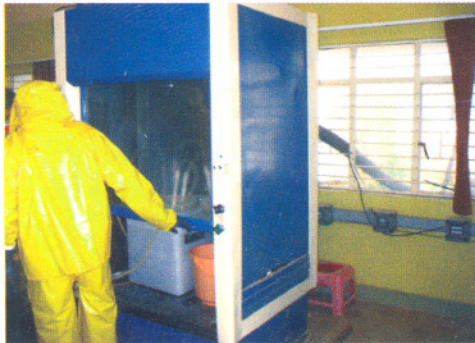
Fig. A.4.1: Experimental set up for BCP of Niobium
