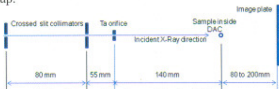
Figure A.2.1: Schematic of setup for the high pressure setup.
